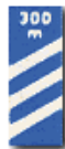
300 Meters to Exit Number of Bars Decreases with Distance; Each Bar Represents 100 Meters
